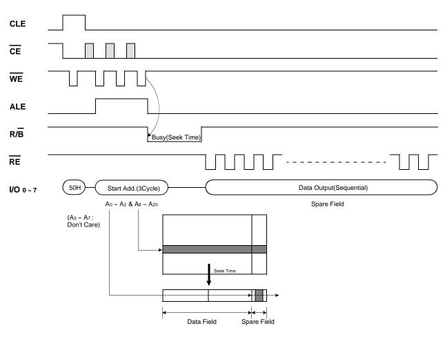
Figure 5. Sequential Row Read1 Operation
