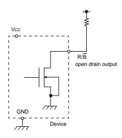
$$Rp = \frac{Vcc(Max.) - VoL(Max.)}{IoL + \Sigma IL} = \frac{Note^*}{8mA + \Sigma IL}$$
