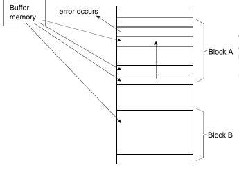
When the error happens in Block "A", try to reprogram the data into another Block "B" by reloading from an external buffer. Then, prevent further system access to Block "A"(by creating a "bad block" table or other appropriate scheme.)
