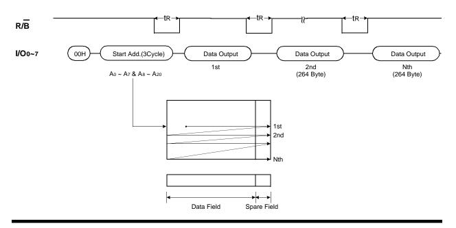
Figure 6. Sequential Row Read2 Operation
