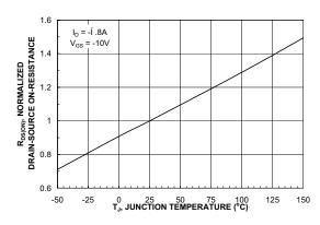
Figure 3. On-Resistance Variation with Temperature.
