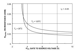
Figure 4. On-Resistance Variation with Gate-to-Source Voltage.
