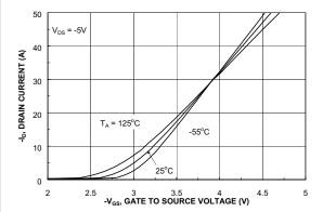
Figure 5. Transfer Characteristics.
