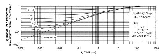
Figure 11. Transient Thermal Response Curve.
