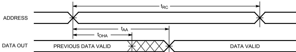
Figure 2 shows  $\overline{OE}$  controlled read cycle waveforms.<sup>[20, 21]</sup>
