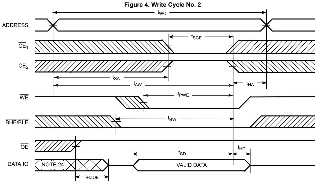
Figure 5 shows  $\overline{WE}$  controlled,  $\overline{OE}$  LOW write cycle waveforms.<sup>[23]</sup>
