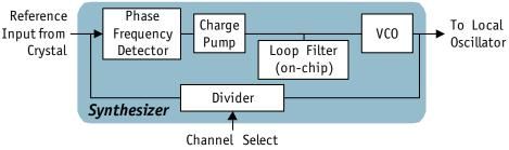
Figure 3-3. Radio Synthesizer Block Diagram
