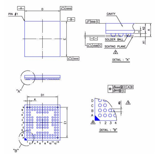
Figure 7-1. BGA Drawing 7 x 7 mm Package
