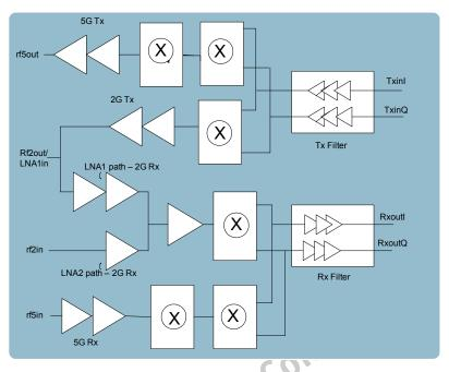
Figure 3-2. Radio Tx/Rx Block Diagram
