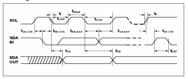
Figure 2 · SCL: Serial Clock, SDA: Serial Data I/O
