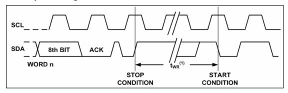
Figure 3. SCL: Serial Clock, SDA: Serial Data I/O
