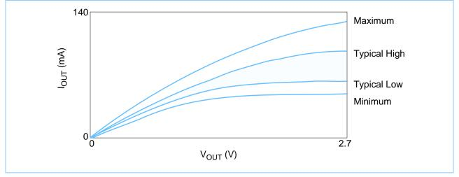
3. The full variation in driver pullup current from minimum to maximum process, temperature and voltage will lie within the outer bounding lines of the V-I curve.
