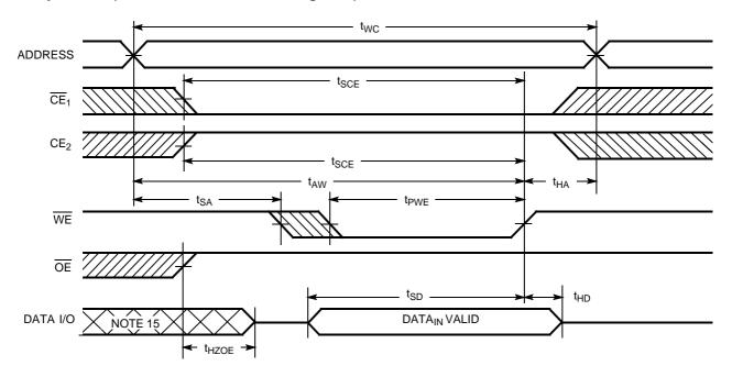
Notes: 13. Data I/O is high impedance if  $\overline{OE} = V_{IH}$ . 14. If  $\overline{CE}_1$  goes HIGH or  $CE_2$  goes LOW simultaneously with  $\overline{WE}$  going HIGH, the output remains in a high-impedance state. 15. During this period the I/Os are in the output state and input signals should not be applied.
