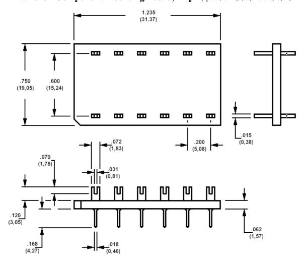
How to order code  $\underline{702-3732-01}$ - $\underline{XX}$ - $\underline{00}$  Basic Part No  $\underline{XX}$  = Plating Finish
