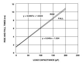
Figure 39. Typical Output Rise/Fall Time (20%-80%,  $V_{DDEXT} = Max$ )
