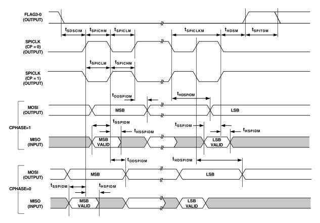
Figure 33. SPI Master Timing
