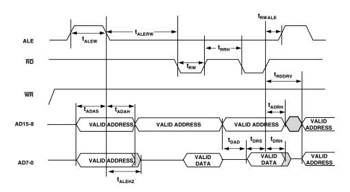
Figure 17. Read Cycle For 8-Bit Memory Timing
