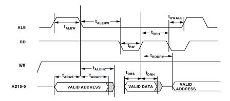
Figure 18. Read Cycle For 16-Bit Memory Timing
