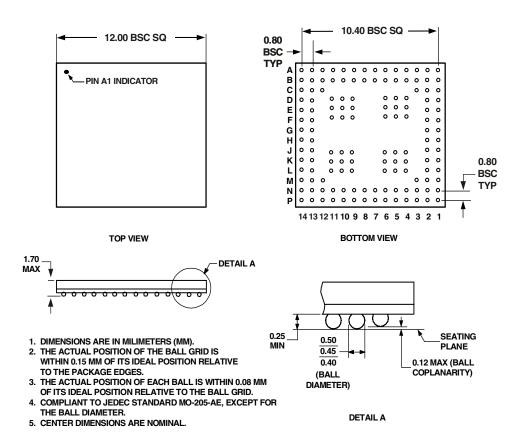
Figure 43. 136-ball Mini-BGA (BC-136-2)
