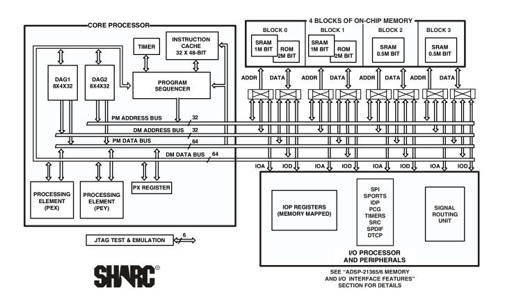
Figure 1. Functional Block Diagram – Processor Core
