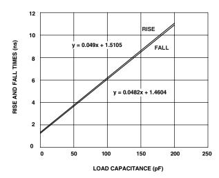
Figure 40. Typical Output Rise/Fall Time (20%-80%, V<sub>DDEXT</sub>=Min)
