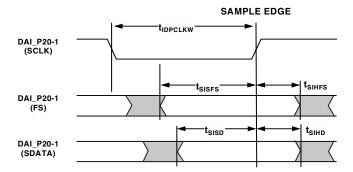
Figure 25. SRC Serial Input Port Timing
