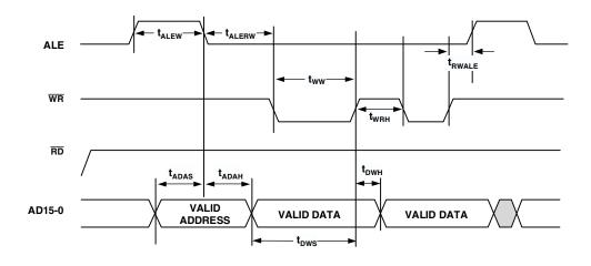
Figure 20. Write Cycle For 16-Bit Memory Timing
