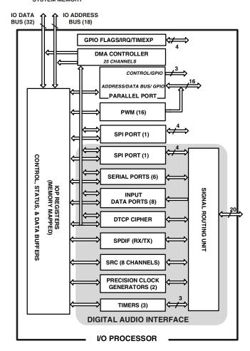
Figure 3. ADSP-21365/6 I/O Processor and Peripherals Block Diagram
