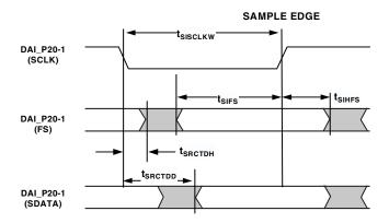
Figure 26. SRC Serial Output Port Timing
