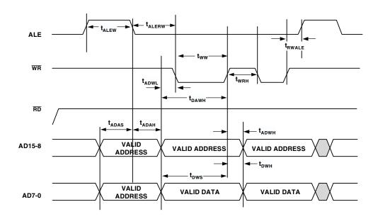
Figure 19. Write Cycle For 8-Bit Memory Timing
