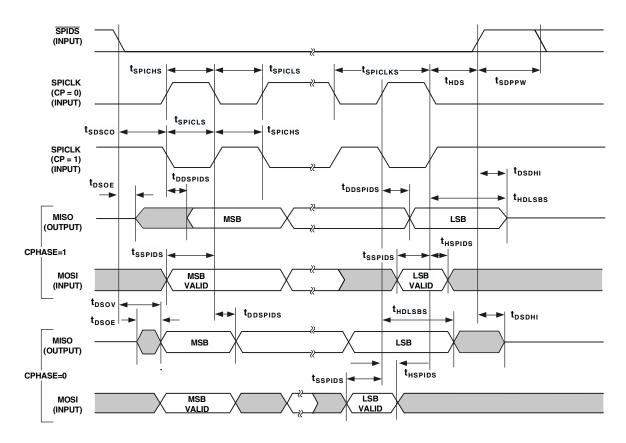
Figure 34. SPI Slave Timing
