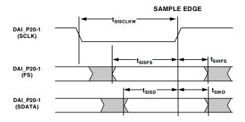
Figure 30. SPDIF Transmitter Input Timing
