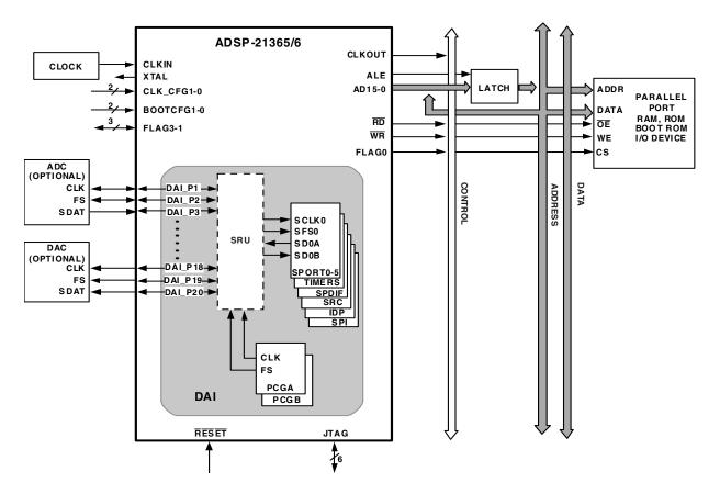
Figure 2. ADSP-21365/6 System Sample Configuration
