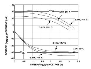
Figure 36. ADSP-21365/6 Typical Drive
