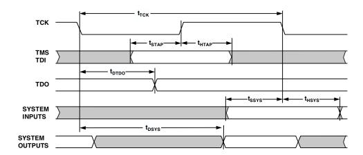
Figure 35. IEEE 1149.1 JTAG Test Access Port
