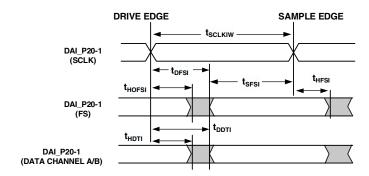
Figure 31. SPDIF Receiver Internal Digital PLL Mode Timing
