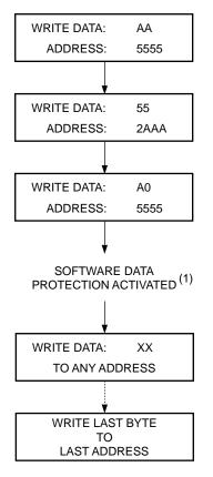
Figure 10. Write Sequence for Deactivating Software Data Protection
