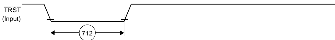
Figure 29. \overline{\text{TRST}} Timing Diagram
