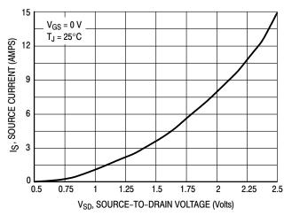
Figure 10. Diode Forward Voltage versus Current
