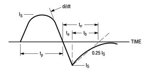
Figure 15. Diode Reverse Recovery Waveform
