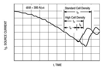
Figure 11. Reverse Recovery Time (t<sub>rr</sub>)
