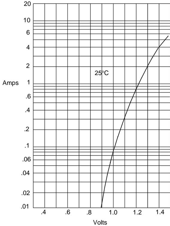
Instantaneous Forward Current - Amperes *versus*
