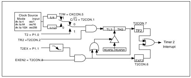
Figure 15. 16-Bit Auto-reload Mode, Counting Up
