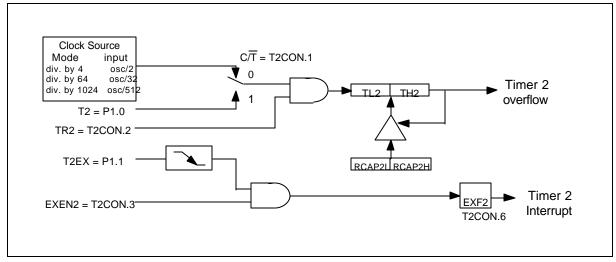
Figure 17. Baud Rate Generator Mode
