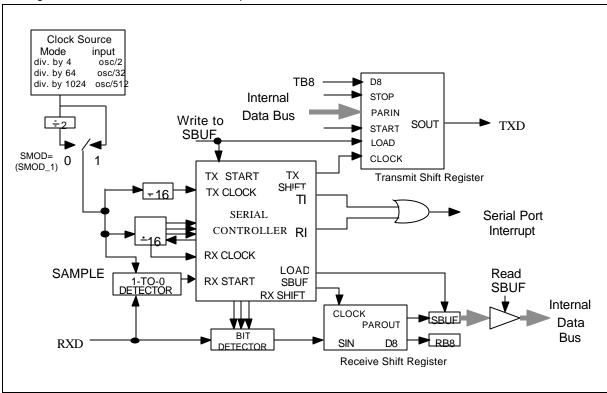
Figure 22. Serial Port Mode 2
