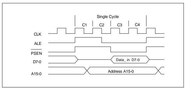
Figure 3. Single Cycle Instruction Timing
