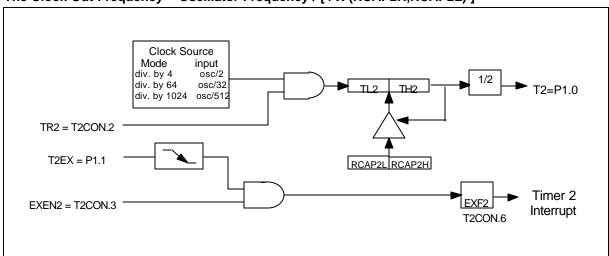
Figure 18. Programmable Clock-Out Mode
