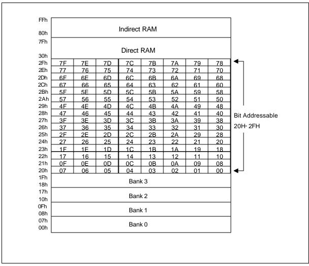
Figure 2. Scratchpad RAM/Register Addressing
