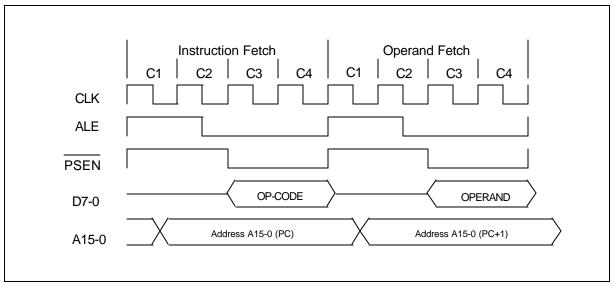
Figure 4. Two Cycle Instruction Timing
