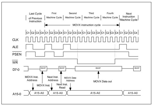
Figure 10. Data Memory Write with Stretch Value = 2
