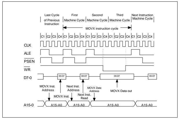
Figure 9. Data Memory Write with Stretch Value = 1
