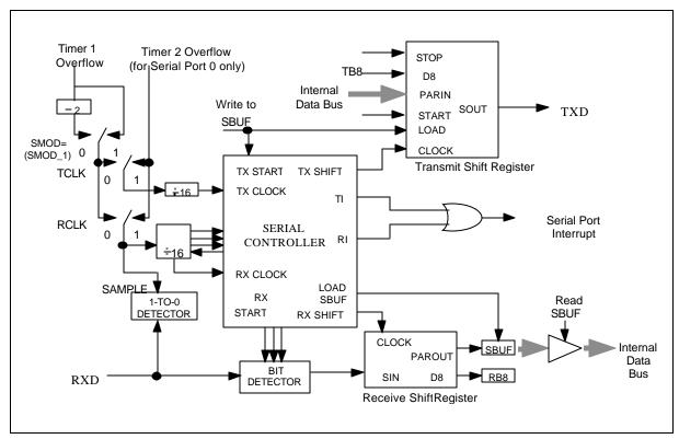
Figure 23. Serial Port Mode 3
