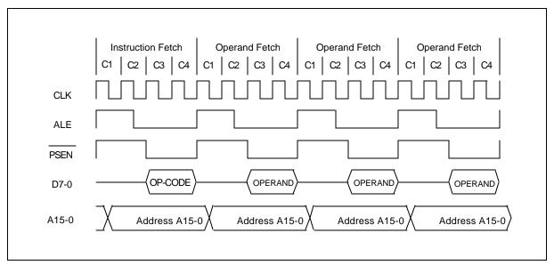
Figure 6. Four Cycle Instruction Timing
