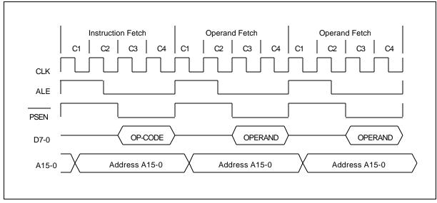
Figure 5. Three Cycle Instruction Timing
