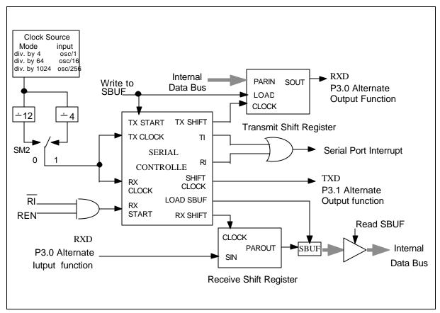
Figure 20. Serial Port Mode 0
