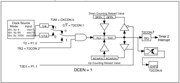
Figure 16. 16-Bit Auto-reload Up/Down Counter
