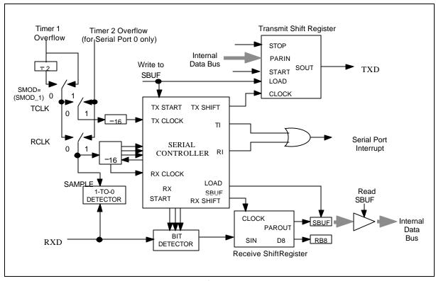
Figure 21. Serial Port Mode 1
