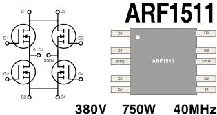
FULL-BRIDGE380V750W40MHzThe ARF1511 is four RF power transistor arranged in an H-Bridge configuration. It is intended for off-line 300V operationin high power scientific, medical and, industrial RF power generator and amplifier applications up to 40 MHz.
