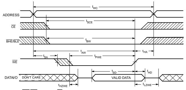
Write Cycle 4 (BHE/BLE Controlled, OE LOW)<sup>[18, 19]</sup>
