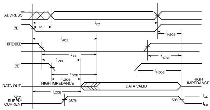
Notes: 15. <u>Dev</u>ice is continuously selected.  $\overline{OE}$ ,  $\overline{CE} = V_{IL}$ . 16. WE is HIGH for Read Cycle.
