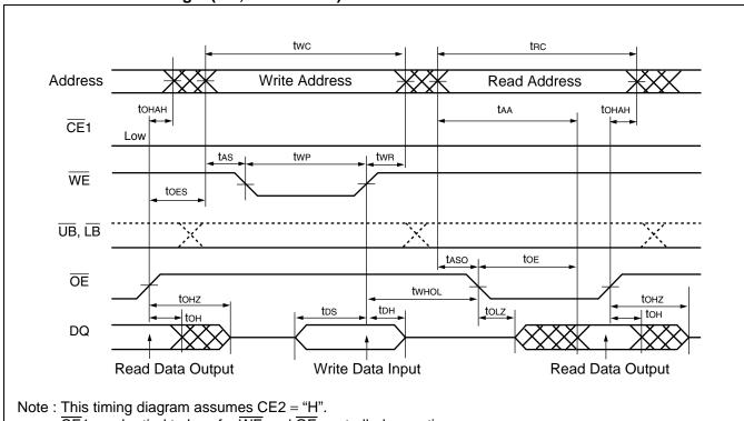
$\overline{\text{CE}}$ 1 can be tied to Low for  $\overline{\text{WE}}$  and  $\overline{\text{OE}}$  controlled operation.
