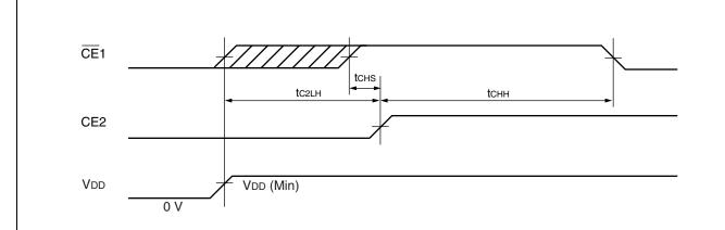
Note: tc2LH specifies after VDD reaches specified minimum level.
