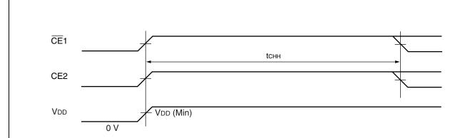
Note: tchh specifies after VDD reaches specified minimum level and applicable to both  $\overline{\text{CE}}1$  and CE2. If transition time of VDD (from 0 V to VDD Min) is longer than 100 ms, POWER-UP Timing#1 must be applied.
