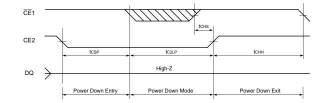
Note: This Power Down mode can be also used as a reset timing if POWER-UP timing could not be satisfied.
