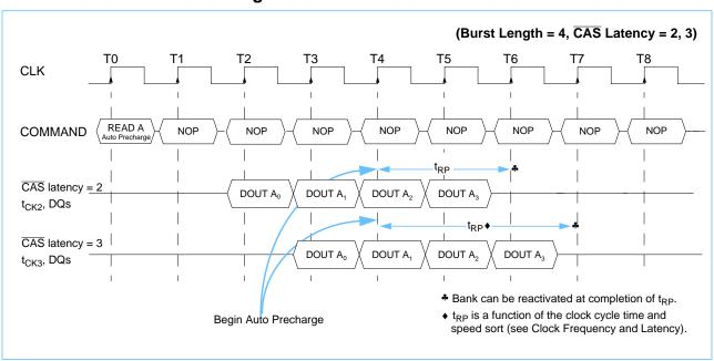
Although a Read command with Auto Precharge cannot be interrupted by a command to the same bank, it can be interrupted by a Read or Write command to a different bank. If the interrupting command is issued before Auto Precharge begins then the Precharge function will begin with the new command.
