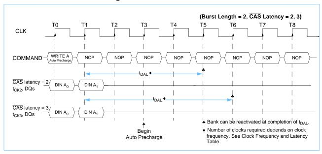
Similar to the Read command, a Write command with Auto Precharge cannot be interrupted by a command to the same bank. It can be interrupted by a Read or Write command to a different bank, however. The interrupting command will terminate the write. The bank undergoing Auto Precharge cannot be reactivated until t<sub>DAL</sub> is satisfied.
