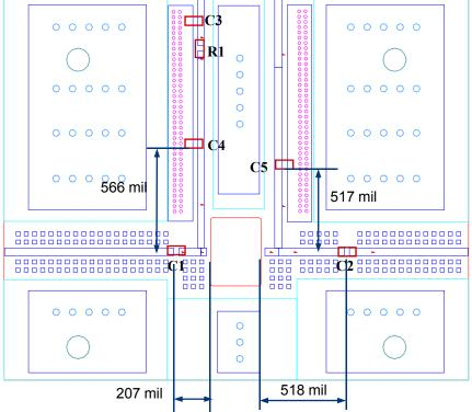
\*The layout is a general purpose drawing that needs to be tuned for the specific application. PCB is RO4003 20 mil thickness, 0.5 oz standard copper cladding, with  $\varepsilon_r$  = 3.38.
