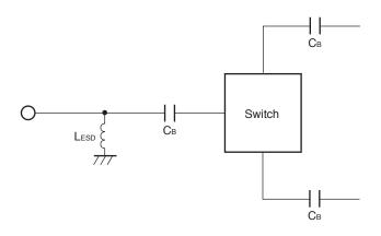
$\bullet$  CB are DC blocking capacitors external to the device.
