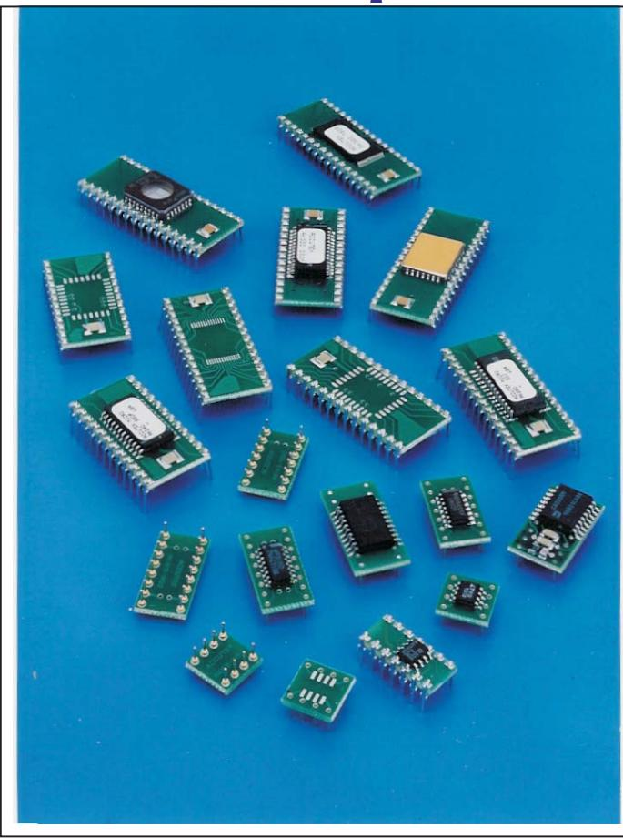
This new family of Accutek DIP Adapter Modules converts surface mount IC's to pin compatible DIP packages for creating drop-in replacements for end-of-life DIP IC's. Package types supported are: SOJ, PLCC, SOIC, SOP, TSOP, QSOP, HSOP, MSOP, LLP (Leadless Leadframe Package), CSP (Chip Scale Package) and CLCC.
