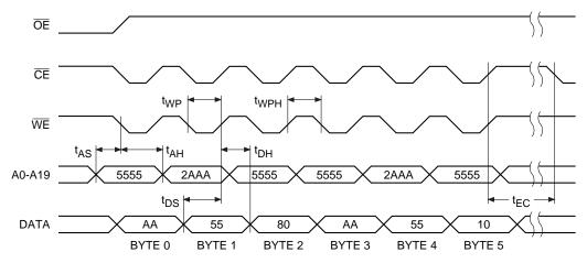
Note:  $\overline{OE}$  must be high only when  $\overline{WE}$  and  $\overline{CE}$  are both low.
