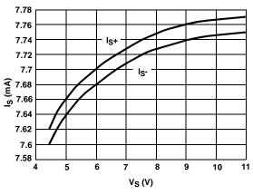
FIGURE 11. SUPPLY CURRENT vs SUPPLY VOLTAGE
