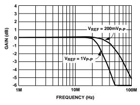
FIGURE 4. FREQUENCY RESPONSE vs  $V_{REF}$
