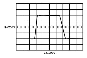
FIGURE 13. V<sub>COM</sub> TRANSIENT RESPONSE
