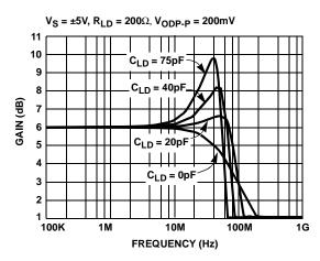
FIGURE 3. SMALL SIGNAL FREQUENCY RESPONSE vs CLD
