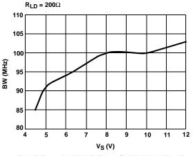
FIGURE 10. BANDWIDTH vs SUPPLY VOLTAGE
