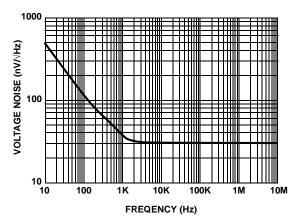
FIGURE 8. INPUT VOLTAGE NOISE vs FREQUENCY
