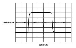
FIGURE 15. SMALL SIGNAL TRANSIENT RESPONSE
