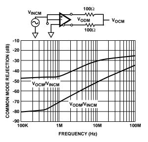
FIGURE 6. COMMON MODE REJECTION vs FREQUENCY
