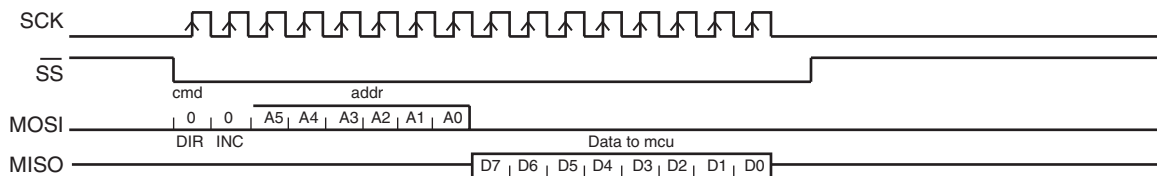
Figure 3-1. SPI Single Read Sequence
