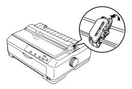
Slide the left sprocket approximately 0.5 inch (12 mm) from the far left position and push the blue lever back to lock it in place. Then slide the right sprocket to match the width of your paper, but do not lock it.
