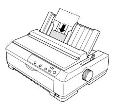
□ Before printing, turn on the card mode by pressing the Tear Off/Bin button several times until the left Tear Off/Bin light is on.
