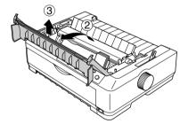
2. Remove the paper tension unit by pressing the tabs on each side and pulling it up.
