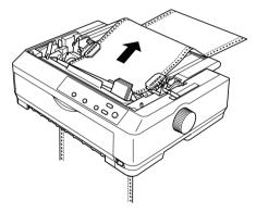
7. Fit four holes of the paper over the tractor pins on both sprockets. Then close the sprocket covers.
