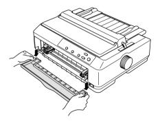
7. Make sure your paper has a clean, straight edge. Then open both sprocket covers and fit the first four holes of the paper, with the printable side up, over the tractor pins.
