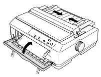
12. Turn on the printer. When the printer receives data, it automatically loads the paper and starts printing.
