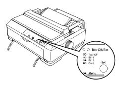
3. Open the paper guide cover, then press the LF/FF ➡ button to feed paper backward, or press the LOGD/Eject ★ button to feed paper forward, until the paper perforation is aligned with the tear-off edge of the printer cover.
