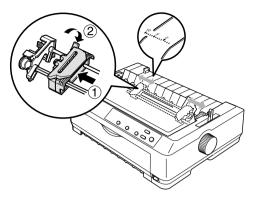
The triangle mark on top of the printer indicates the point furthest to the left where printing can begin.
