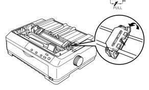
Slide the left sprocket approximately 0.5 inch (12 mm) from the far left position and push the lever back to lock it in place.
