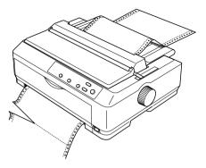
2. To feed paper forward and eject it, hold down the LF/FF button.
