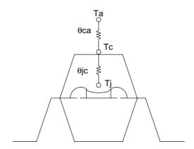
Figure 3.1 Thermal Resistance of Package
