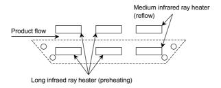
Figure 3.2 Heating Top and Bottom with Long or Medium Infrared Rays
