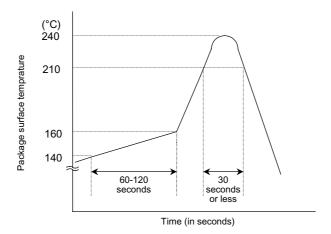
Figure 3.3 Sample Temperature Profile for Infrared or Hot Air Reflow
