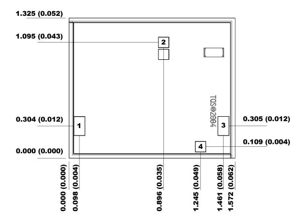
Units: millimeters (inches) Thickness: 0.100 (0.004) Chip edge to bond pad dimensions are shown to center of bond pad Chip size tolerance: +/- 0.051 (0.002)
