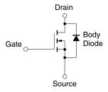
**Remark** Strong electric field, when exposed to this device, can cause destruction of the gate oxide and ultimately degrade the device operation. Steps must be taken to stop generation of static electricity as much as possible, and quickly dissipate it once, when it has occurred.
