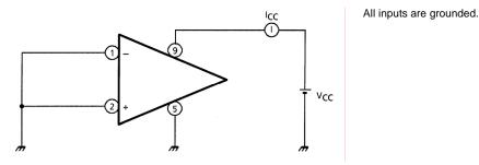
Note: The components illustrated in the test circuit diagrams are intended only to confirm device characteristics.
