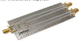
The unbalanced port return loss plot was measured at the input of the aforementioned test board. Unbalanced port
