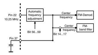
For fine tuning, the center frequency of all these integrated active filters (band filter and demodulator) can be shifted in steps of 6.25 kHz by means of bit 56 to bit 59. Additionally, the center frequency of the band filter can be adjusted separately by means of bit 14 to bit 17.
