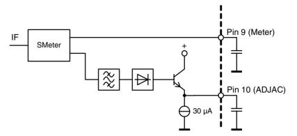
MPINT and ADJAC Reset Bit 6 allows a resets of the multipath sensor and the adjacent channel sensor by connecting pin 10 and pin 40 internally to ground and so the external capacitors can be discharged very quickly.
