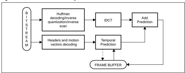
Figure 1 shows the block diagram of the Main Profile decoder [1]. The basic building blocks are the same as for Simple Profile, but some additional features are supported in Main Profile. In particular, Main Profile defines a new type of pictures, called B (bidirectionally interpolated), that are predicted from past and future I/P images. This implies an increased complexity of the *Temporal Prediction* block to support bidirectional prediction.
