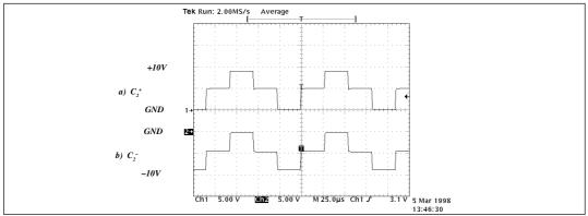
Figure 3. Charge Pump Waveforms
