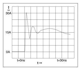
Figure 8. ESD Test Waveform for IEC1000-4-2
