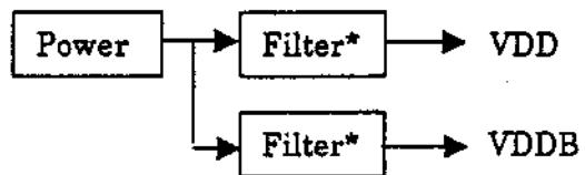
$\left[ \begin{array}{l} \text{Filter*}(\text{reference value}) \\ L = 10 \mu\text{H to } 100 \mu\text{H} \\ C = 10 \mu\text{F to } 100 \mu\text{F} \end{array} \right]$
