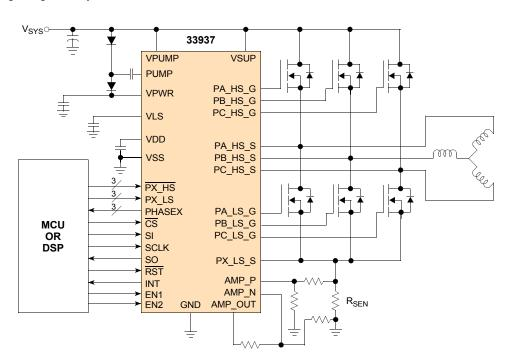
Figure 1. 33937 Simplified Application Diagram
