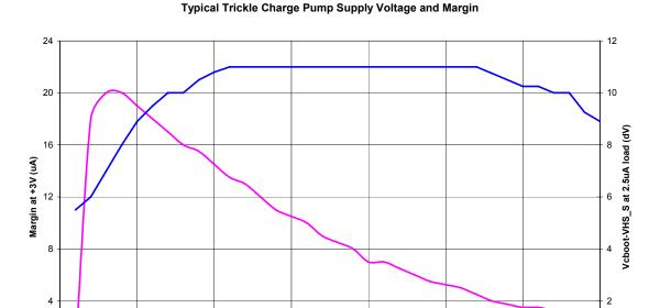
Figure 11. Typical Trickle Charge Pump Supply Voltage and Current Margin vs Supply Voltage
