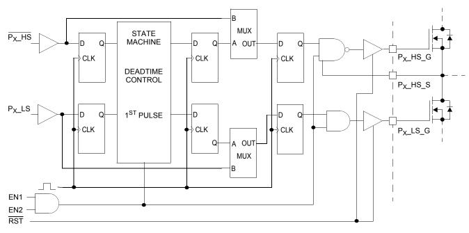
Figure 6. Deadtime Control Delays
