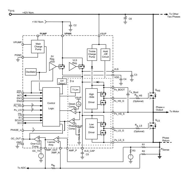
Figure 23. High Voltage Application Diagram (+42 V Battery System)
