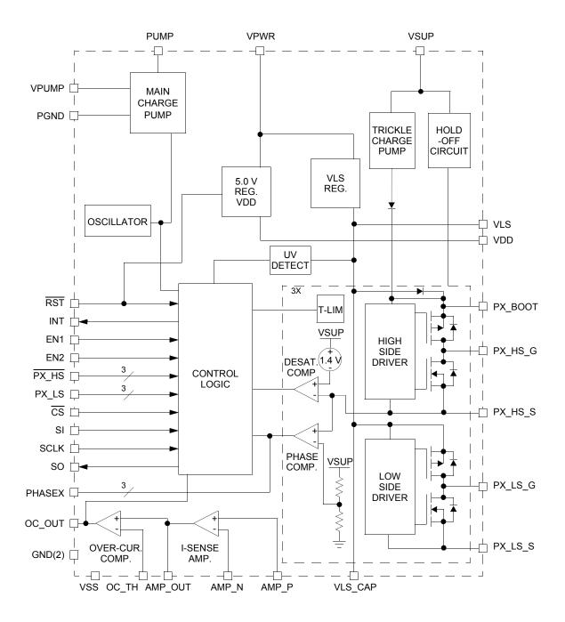
Figure 2. 33937 Simplified Internal Block Diagram
