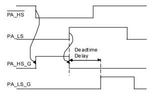
Figure 16. Edge Sensitive Logic Inputs (Phase A)
