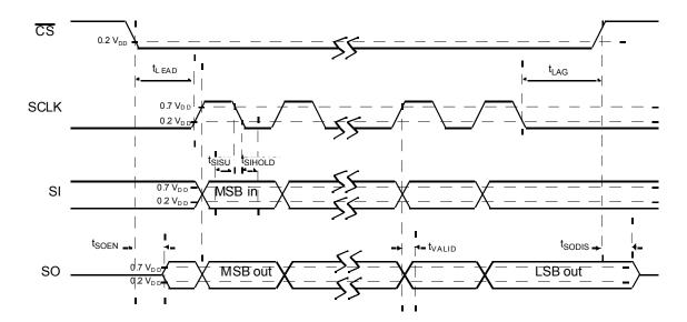
Figure 4. SPI Interface Timing
