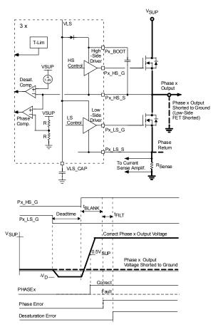
Figure 18. Short to Ground Detection
