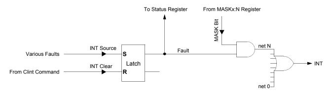
Figure 20. Interrupt Handling
