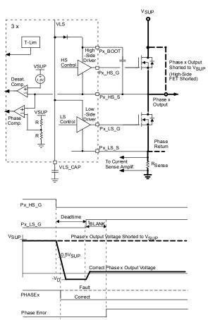
Figure 19. Short to Supply Detection
