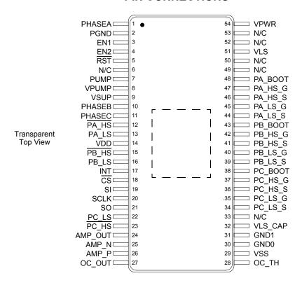
Figure 3. 33937 Pin Connections
