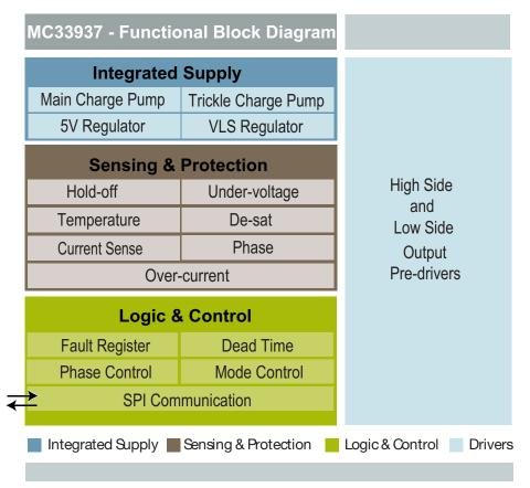
Figure 15. Functional Internal Block Description
