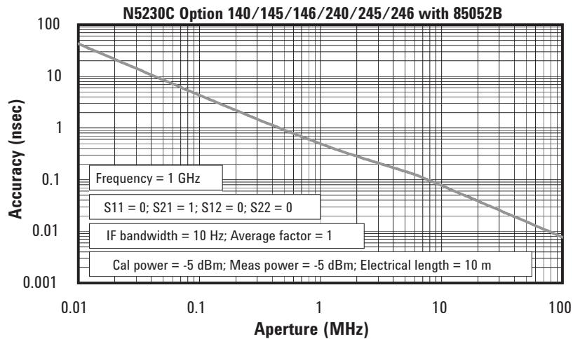
In general, the following formula can be used to determine the accuracy, in seconds, of specific group delay measurement:
