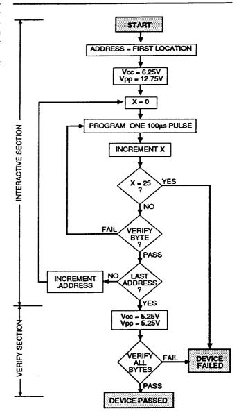
NOTE: THE ALGORITHM SHOWN HERE MUST BE USED TO ENSURE CORRECT PROGRAMMING OF THE PUMA 2U8002. THIS MAXIMIZES THE DATA RETENTION TIME OF THE UV EPROMS AND DOES NOT STRESS THE MEMORY CELL.
