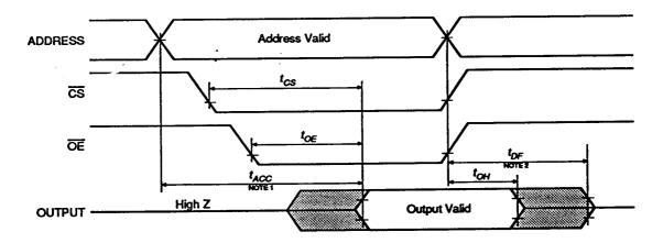
Notes: (1)  $\overline{OE}$  may be delayed up to  $t_{acc}$ - $t_{oe}$  after the falling edge of  $\overline{CS}$  without impact on  $t_{acc}$ .
