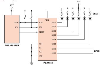
The LED Dimmers feature open drain outputs that sink 25 mA per bit with a maximum of 50 mA for the PCA9530, 100 mA for the PCA9531/33 and 200 mA (100 mA per 8-bit group) for the PCA9532.
