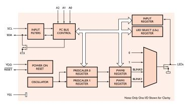
The PCA9530/31/32/33 functional diagram and I/O schematic are identical except for the number of bits and address pins.
