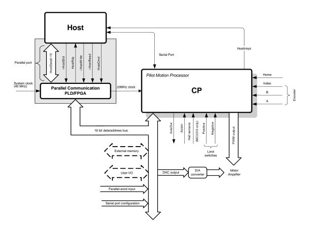
The shaded area shows the CPLD/FPGA that must be provided by the designer if parallel communication is required. A description and the necessary logic (in the form of schematics) of this device are detailed in section 6 of this manual. The CP chip contains the profile generator, which calculates velocity, acceleration, and position values for a trajectory; and the digital servo filter, which stabilizes the motor output signal.
