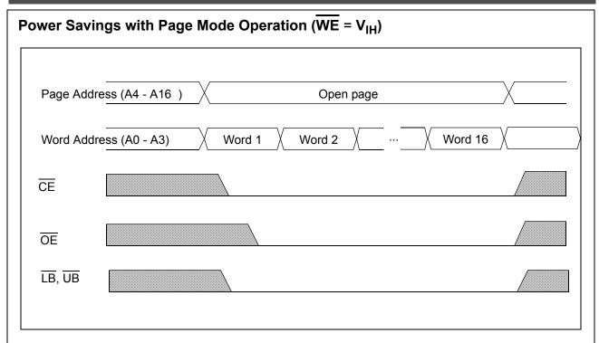
Note: Page mode operation is a method of addressing the SRAM to save operating current. The internal organization of the SRAM is optimized to allow this unique operating mode to be used as a valuable power saving feature.
