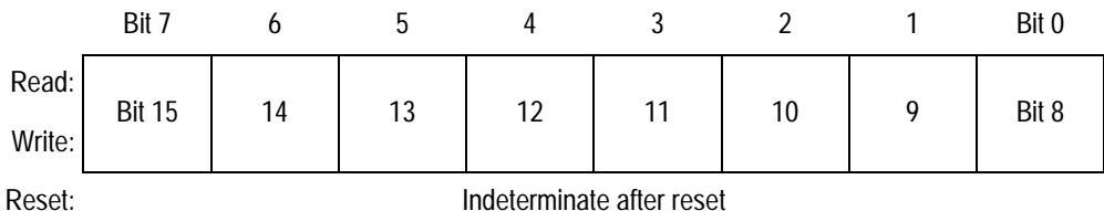
Figure 22-16. TIM Channel 1 Register High (TCH1H)
