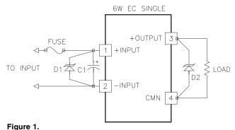
Standard connections for the 6 Watt EC Single. The input fuse should not be omitted. The overvoltage diodes D1 and D2 may be added to the circuit directly at the converter to provide transient protection to your circuit. In some circuits capacitor C1 may be required, see the section "Applying The Input" for more information.
