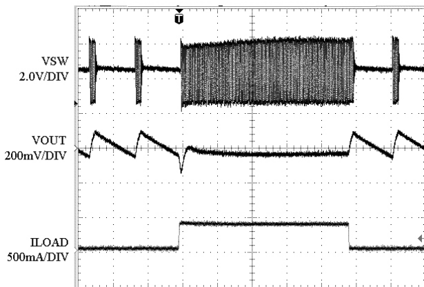
Iload = 26 mA TO 400 mA, Power Saving Mode to PWM Mode L=2.2uH, Cin=10uF, Cout=10uF, Vin=3.6V, Vout=1.8V
