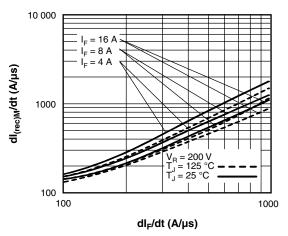
Fig. 8 - Typical  $dI_{(rec)M}/dt$  vs.  $dI_F/dt$
