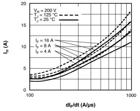
Fig. 6 - Typical Recovery Current vs. dI<sub>F</sub>/dt
