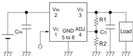
R<sub>1</sub>, R<sub>2</sub>: Output voltage setting resistorsThe output voltage can be set by connecting R<sub>1</sub> and R<sub>2</sub> as shown above.The recommended value of R<sub>2</sub> is 24 kΩ.
