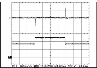
Figure 12: Output voltage response to step-change in load current (50%-75%-50% of lout(max):  $dI/dt = 5A/\mu s$ ). Load cap:  $480\mu F$ ,  $15 \text{ m}\Omega$  ESR tantalum cap and  $1\mu F$  ceramic cap. Top trace: Vout (200mV/div), Bottom trace: lout (10A/div).
