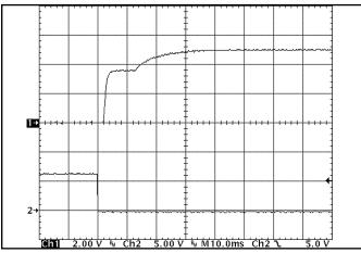
Figure 9: Turn-on transient at full load (resistive load) (10 ms/div). Input voltage pre-applied. Top Trace: Vout (2V/div). Bottom Trace: ON/OFF input (5V/div).
