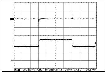
**Figure 11:** Output voltage response to step-change in load current (50%-75%-50% of Iout(max);  $dI/dt = 0.1A/\mu s$ ). Load cap:  $15\mu F$ ,  $450 \text{ m}\Omega$  ESR tantalum cap and  $1\mu F$  ceramic cap. Top trace: Vout (200mV/div), Bottom trace: Iout (10A/div).
