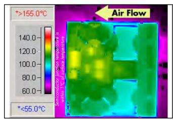
Figure 8: Thermal plot of converter at 40 amp load current with 55°C air flowing at the rate of 200 LFM. Air is flowing across the converter from output to input (nominal input voltage).
