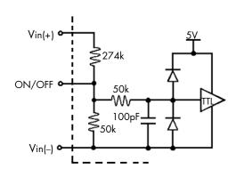
Figure B: Internal ON/OFF pin circuitry
