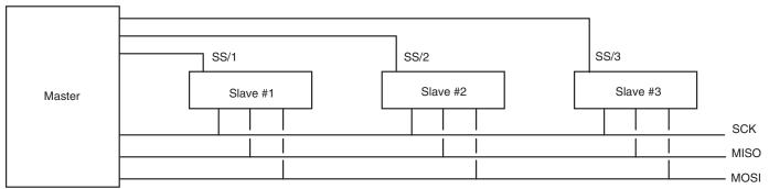
When a master is connected with several slaves, the signals SCK, MISO and MOSI are interconnected. Each slave SS/ is driven separately. Only one slave can be selected, the others have their MISO tri-stated and ignore MOSI data.
