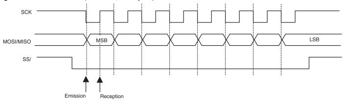
Note: During initialization of the SCK wire (power-on or reset), SS/ has to be inactive ('1').
