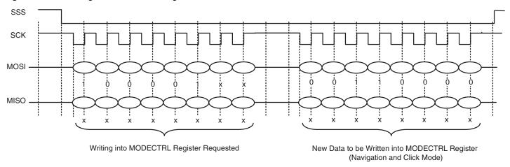
Note: The break on SCK on the SPI chronogram has been added for better comprehension only. In a real application, SCK can be continuous.
