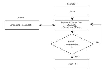
During an 8-bit access, the sensor transmits two pixels (each pixel is coded on 4 bits).
