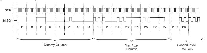
Notes: 1. For the first array or frame reading, 40 dummy clock cycles must be sent before the first data arrives. This is necessary for the initialization of the chip pipeline. Consequently, the first synchronization sequences appear after 40 clock cycles. For the following array readings, data arrives at each clock cycle. One should implement a synchronization routine in the protocol to look for the F0F00200 pattern.
