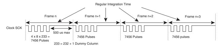
Note: The 500 µs duration corresponds to the host's computation time (slice reconstruction, finger detection...) and in the illustration is given as an example only. Once the host detects a finger, this value remains constant, thus guaranteeing a regular integration time.
