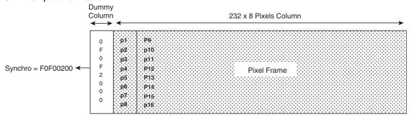
The first dummy column, at the beginning of the pixel array, is added to the sensor to act as a specific easy-to-detect pattern, and represents the start of the frame tag.
