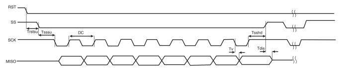
Figure 7-2. Read/Write Timing Slow SPI Slave Mode
