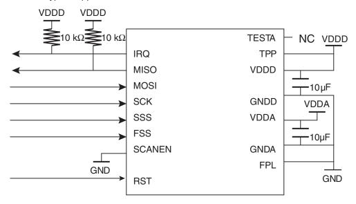
The pull-up must be implemented for the master controller. The noise should be lower than 30 mV peak-to-peak on VDDA and VDDD.
