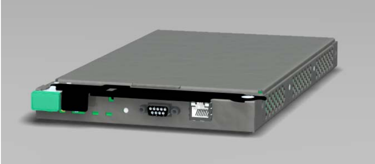
Figure 18. Front View of Chassis Management Module
