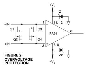
versals or opens on the negative supply rail is known to induce input stage failure. Unidirectional transzorbs prevent this, and it is desirable that they be both electrically and physically as close to the amplifier as possible.
