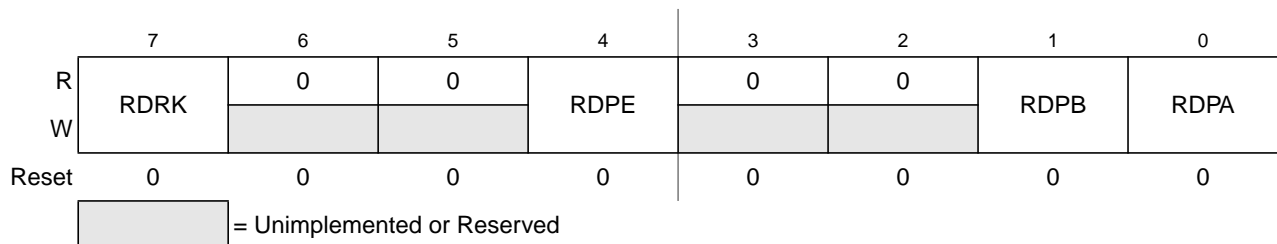
Figure 18-15. Reduced Drive Register (RDRIV)
